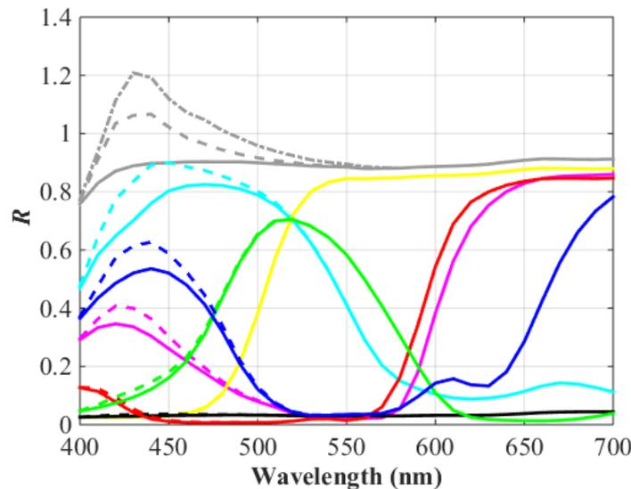
Figure 1. Measured reflectance factors  $R$  of the process inks and paper without fluorescence (solid) and simulated  $R$  with fluorescence in illuminant CIEA (dash) and CIED65 (dash-dot, only bare paper). The inks are represented by their respective colours. Note that light tones and ink combinations with only cyan, blue and magenta are the most subject to colour shifts due to fluorescence.
