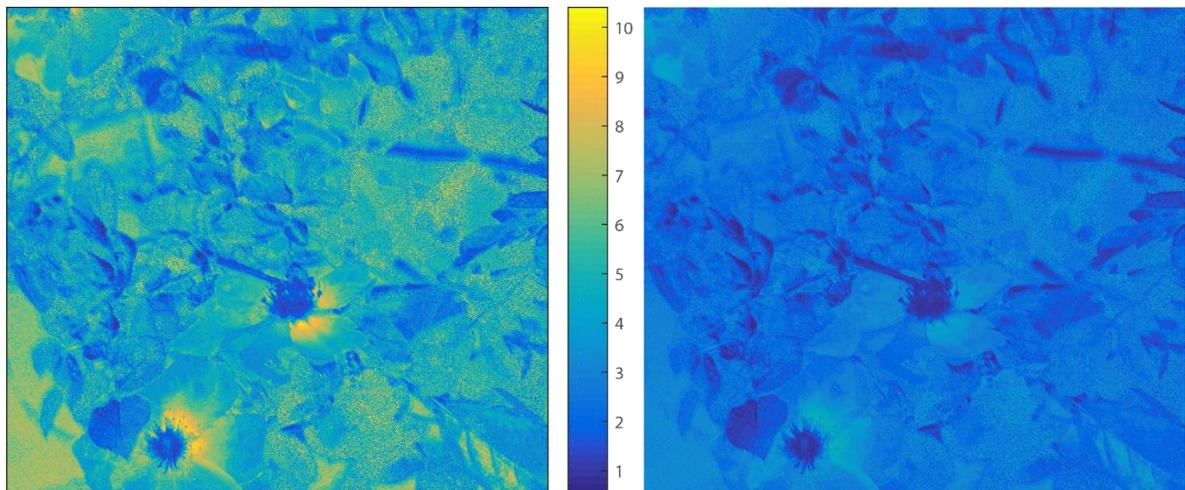
*Figure 3. DE2000 colour-difference maps for CIED65 (left) and CIEA (right). Note that daylight, which contains more energy in the UV wavelengths and therefore engenders more fluorescence, yields colorimetric errors larger than 10 DE2000 for this particular image*
