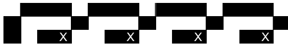
Figure 6. A worst case scenario for stack size. Entries to the stack are noted by “X”
